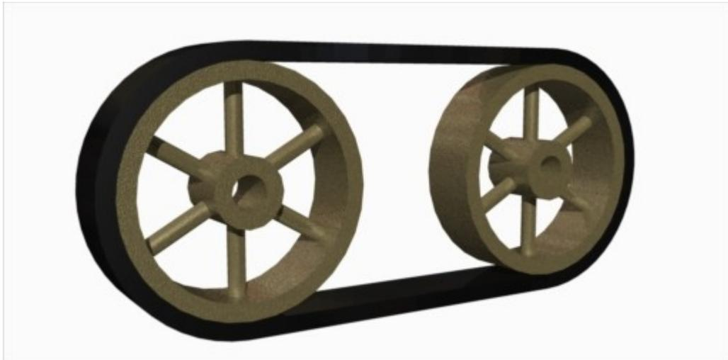
The belt will now appear in the preview window wrapped around the wheels. Adjust the belt width and thickness, in this example the Thickness is 1/2 inch. 3 different belt types are available, flat, v-belt and round. The *Thickness* parameter changes to become the *Diameter* for a round belt. The level of detail adjusts the number of segments used to make up the belt length and the number of points on the cross section for a round belt can also be adjusted.
