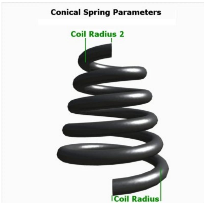
When the Conical spring option is enabled the *Coil Radius 2* sets the radius for the upper most coil of the spring. When a non-zero *From Height*: is set the spring coils keep the main radius until that height is reached. *Currently a From Height > 0 does*
