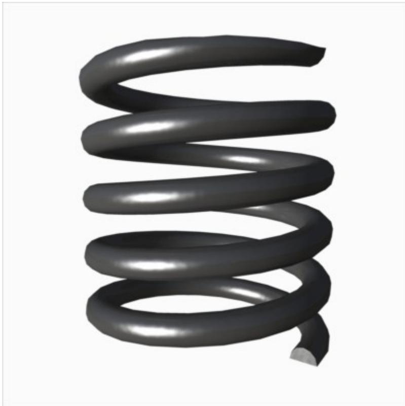
When the option to *Grind Ends* is checked the first and last turns of the spring are created so they present a flat surface.
