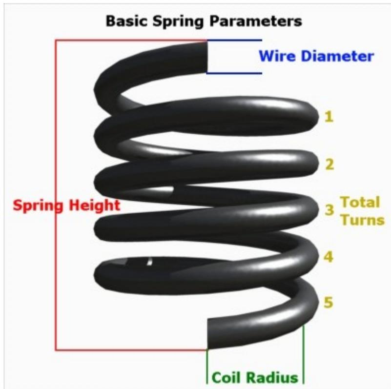
The basic parameters used to describe the spring are simple. Note that the *Coil Radius* is the length from the centre of the spring to the centre of the wire.
