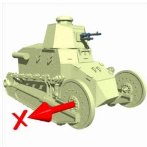
All of the wheels and the pins of the links must have their axles aligned either in the X or Y axis. If the wheels need to be orientated to fit them to the vehicle assembly then group each wheel to preserve the rotation. For this tank the axles are aligned in the X axis and the vehicle faces in the Y axis. The hot point of each wheel should be in the middle of its hub.
